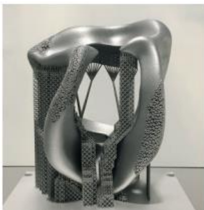
Fig 1: AlSi10Mg demo part manufactured in segments with dynamic adaptive parameter sets. Volume rate: 12 up to 32 mm³/s Source: EOS Innovation Center Düsseldorf
