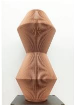
Fig 2: CuCrZr demo part The first ever 1000mm CuCrZr AM part
