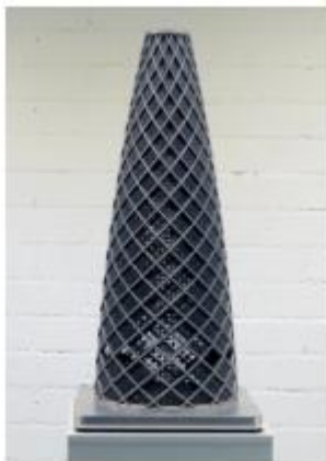
Fig 1: AISi10Mg demo part 1.000mm height, Ø 380mm, Build time: ~ 73 hours
