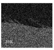
Cladding interface layer XZ Electron Microscopy
